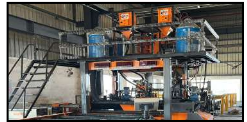
Automatic Gantry Submerged Arch Welding 2
