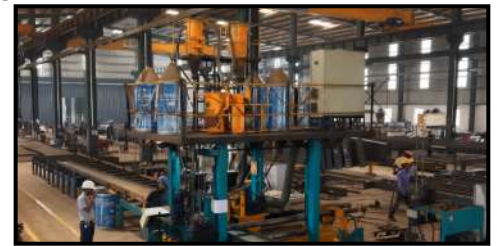
Automatic Gantry Submerged Arch Welding 1
